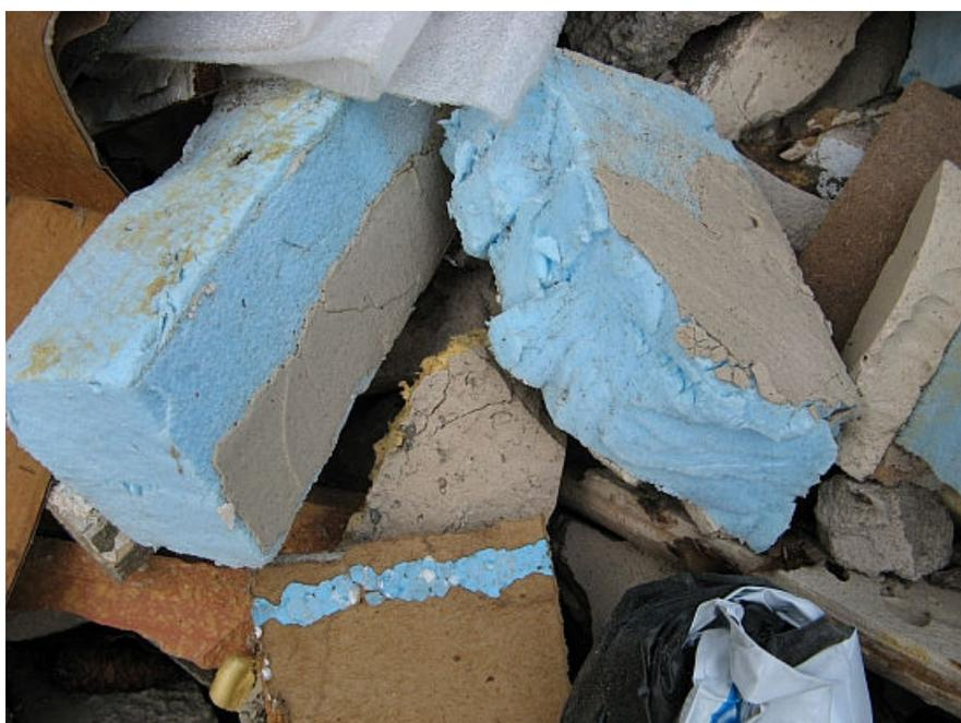
**Figure 17** Construction waste containing different fractions such as concrete or XPS boards (source: Empa)
