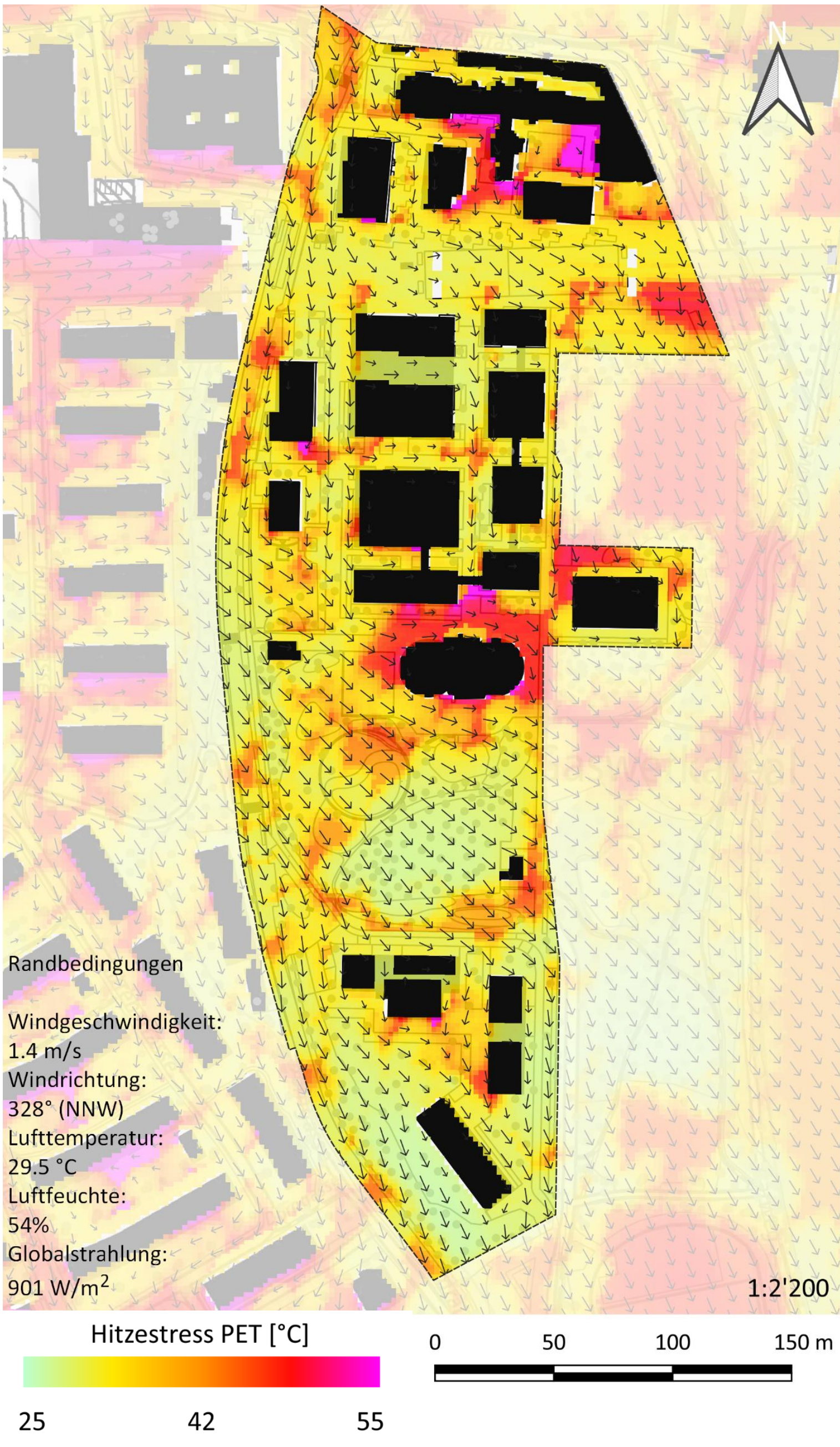
Fig. 3: Heat stress simulation during the day using ENVI-met.
